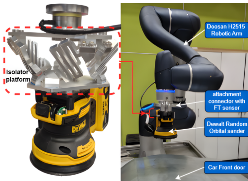
Figure 9: The integrated MAGICIAN grinding tool composed of the Stewart-Based Folded-Beam Passive Vibration Isolator, the FT sensor, and the DeWalt DCW210 grinder.
