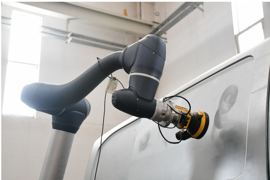
Figure 4: The grinding tool integrated on the Cleaning Robot composed by the ATI FT Mini-45 and the DeWALT DCW210N-XJ 18V XR 125mm grinder.
